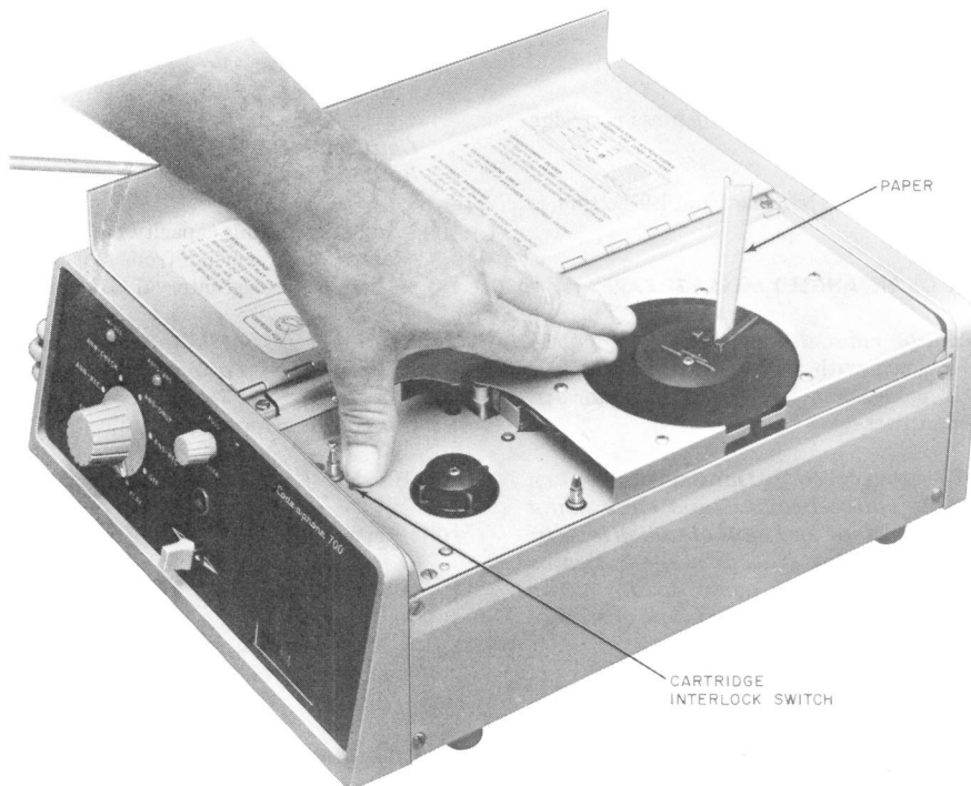
Fig. 7—Resetting “0” Registration on Message Indicator Dial
